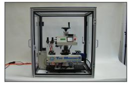
The Sound Enclosure is designed to minimize noise, add operator protection, while providing easy access for machine loading and service. The enclosure features 4 doors, all removable, for access from all sides. Each side has a rubber seal, magnetic latch and large handle. Supplied as a kit with pre-drilled panels, structure elements and hardware for simple assembly with screwdriver and allen keys.
