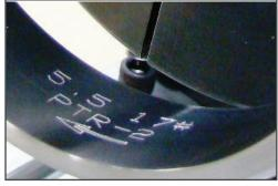
The KT 1000 Inside Diameter marking attachment is designed to address the often "awkward" setup and tooling required to mark the inside surface of rings, tubes, etc. A machine tool quality dual ball slide, with height adjustment, is used to support the marking head while it moves into the ID. The standard KwikTurn 5-C cylindrical attachment is used to rotate the part.
