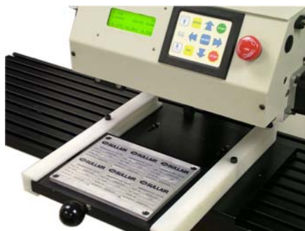
Nametag Nest Quick slide in nest streamlines manually loading the system. Adjustable for size.
